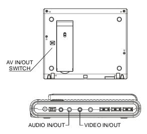
When push the **AV IN/OUT** switch to **IN**, the player will stop normal playback and act as a TFT MONITOR.
